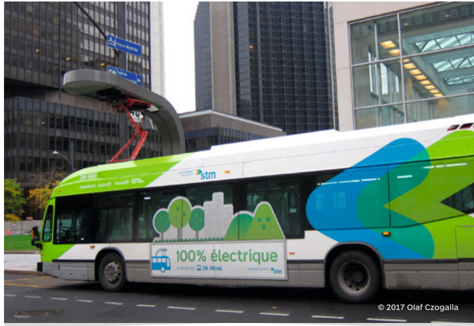
Electric bus parking in a Pantograph charging station in Montreal, Canada
