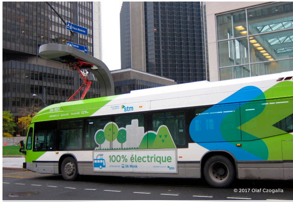
Electric bus parking in a Pantograph charging station in Montreal, Canada
