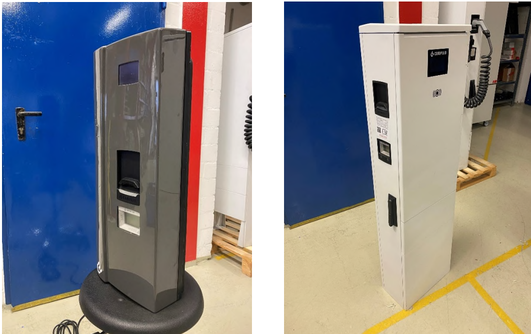
Figure 2: Functional prototypes. Left: Charging station with single charging point, Right: charging station with two charging points.
