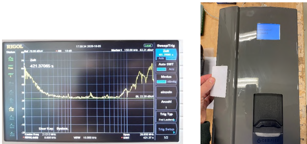
Figure 3: A screenshot of the oscilloscope during an internal EMC test (left) and authorization test via an RFID card (right).
